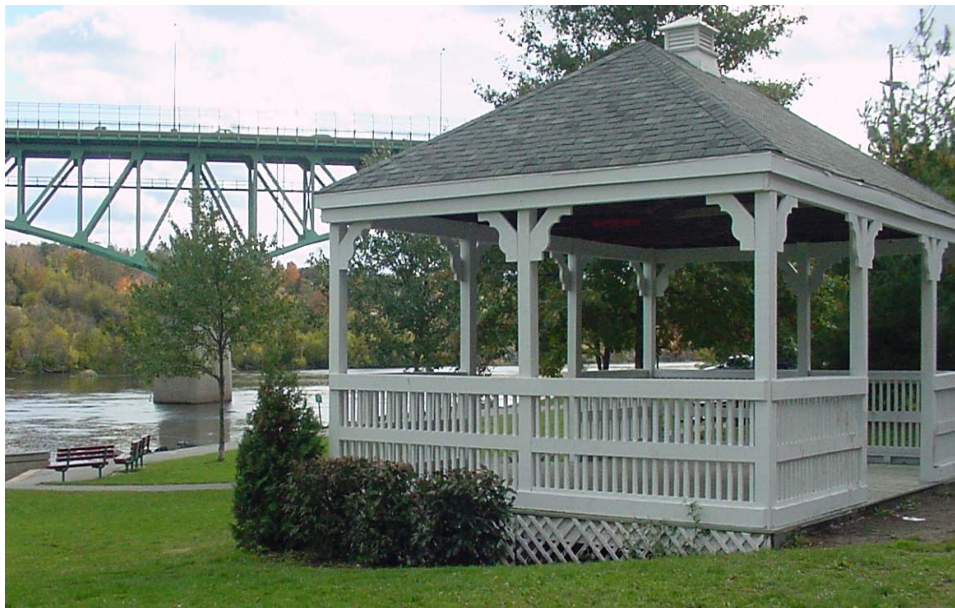
(Augusta, ME) This riverside gazebo is moveable and can be towed out of the floodplain. Photo from the Maine Floodplain Management Program.
